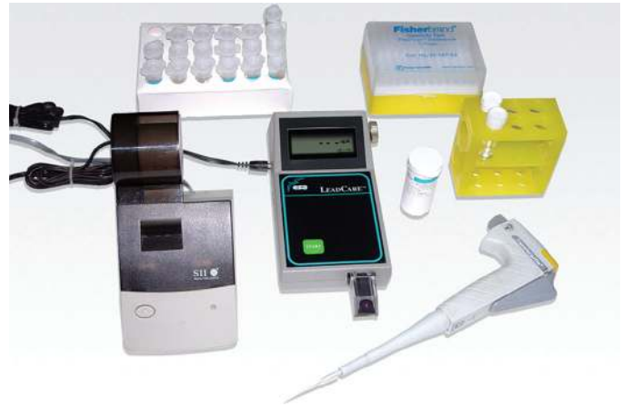
FIGURE 10-27 The LeadCare System is widely used in the diagnosis of lead toxicosis in birds. It relies on electrochemistry and a sensor to detect lead levels in whole blood.
