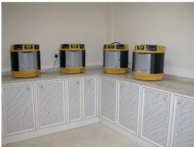
FIGURE 15-40 Brooders are essential to maintaining the necessary environmental conditions for hand-rearing chicks in the first stage of development. The Brinsea TLC 4 parrot brooder is a reliable unit that can be used for a wide variety of species. In tropical and arid countries, it is advisable to place these units over short legs within shallow dishes (e.g., Petri dishes) containing mineral or vegetable oil to prevent ants from climbing into the units and hurting and even killing chicks. (Courtesy Dr. Jaime Samour.)
