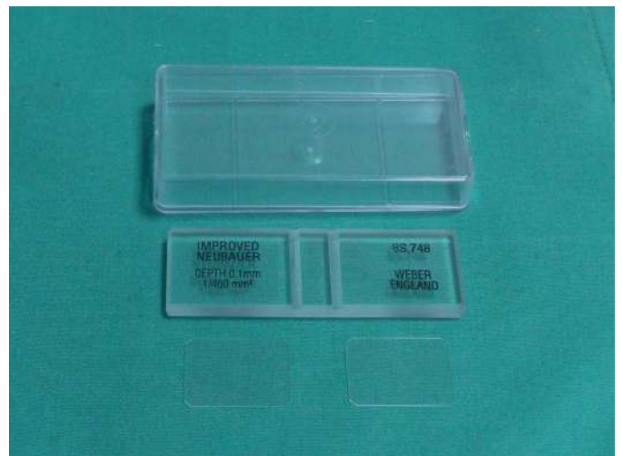
FIGURE 15-20 The Improved Neubauer Counting Chamber has been widely used over the years to determine the spermatozoa concentration in semen samples. (Courtesy Dr. Melodiya Magno.)
