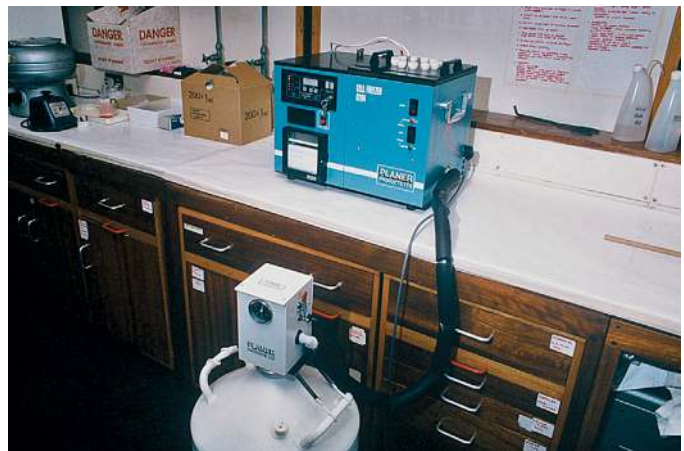
FIGURE 15-32 Programmable cell freezer used successfully for the cryopreservation of semen samples from budgerigar ( Melopsittacus undulatus ). A pump mounted on the top of the liquid nitrogen storage flask propels liquid nitrogen vapor into the loaded freezing chamber according to a designated program.
