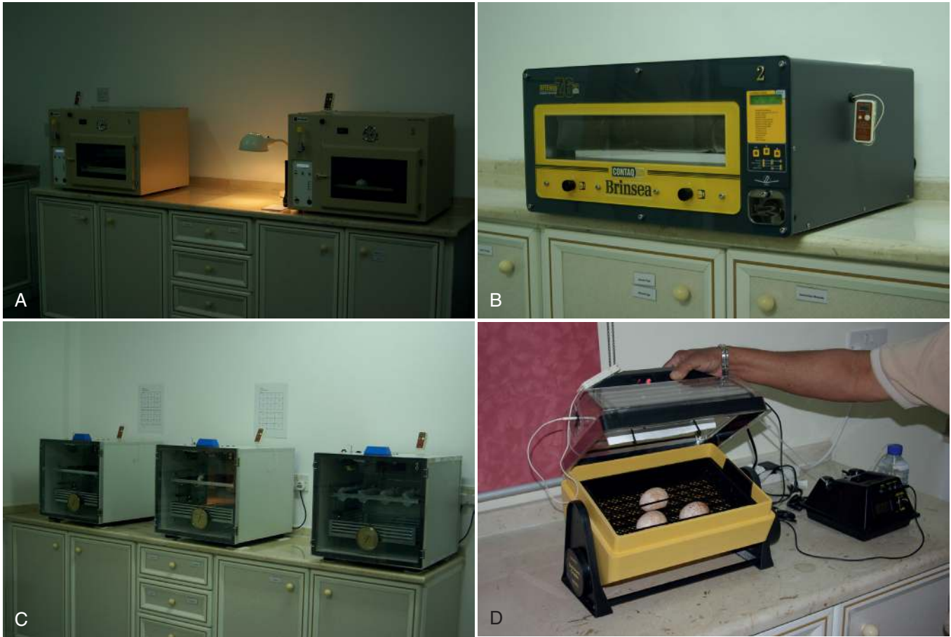
FIGURE 15-34 (A-D) , The images show four types of incubators commonly used for eggs of different avian species. In some of these units, the eggs are placed horizontally over rollers, while in others, the eggs are placed vertically within holders. The incubator in (B) is a “contact” incubator, so called because during incubation the eggs are covered periodically by a plastic membrane simulating the effect of the brood patch of the hen. Many experienced breeders like moving around the eggs of some species using different incubators. Commonly, breeders start the incubation period by setting the eggs in an incubator and placing them horizontally for the first quarter. Later, they transfer the eggs to another incubator, placing them in the vertical position until pipping.
