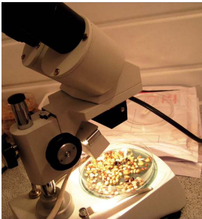
FIGURE 3-8 A key initial part of analysis is microscopic examination. Here a seed sample is investigated for quality using a stereomicroscope.
