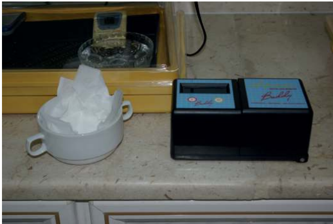
FIGURE 15-37 Electronic egg cardiac monitors (Buddy) are used to assess the heartbeat of embryos from the first quarter of the incubation period. These monitors are used effectively to monitor the embryo's development during incubation and to assess the embryo's health status during the hatching process.
