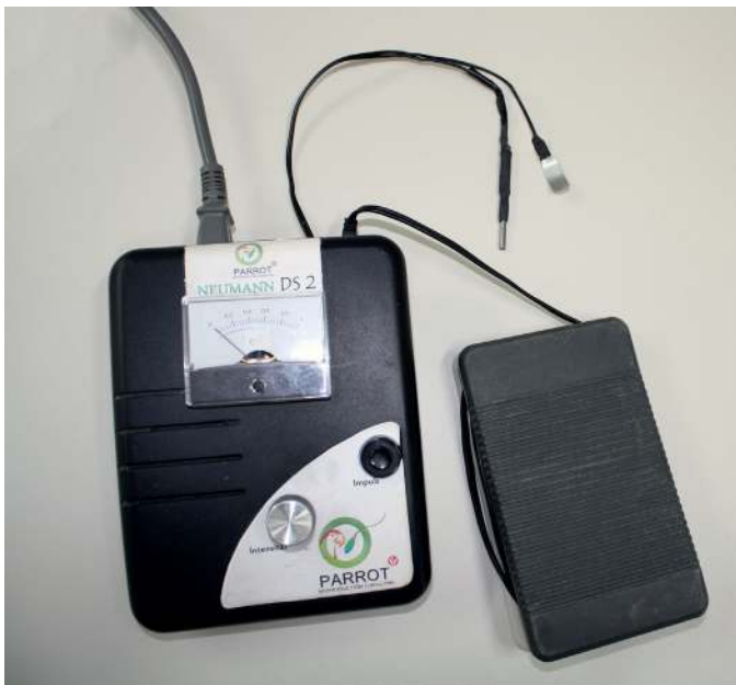
FIGURE 15-18 The main electroejaculation unit consists mainly of a potentiometer, a voltmeter with an analog display of the voltage intensity, and an operating foot pedal to provide hands-free operation of the unit during the semen collection procedure. (Courtesy Parrot Reproduction Consulting.)
