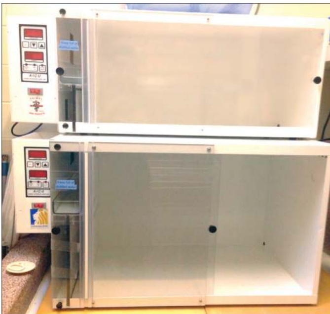
FIGURE 8-14 Animal Intensive Care Unit by Lyon Electric. These incubators come in two sizes, are made of metal, and are stackable. A small opening on the back can accommodate an oxygen line.
