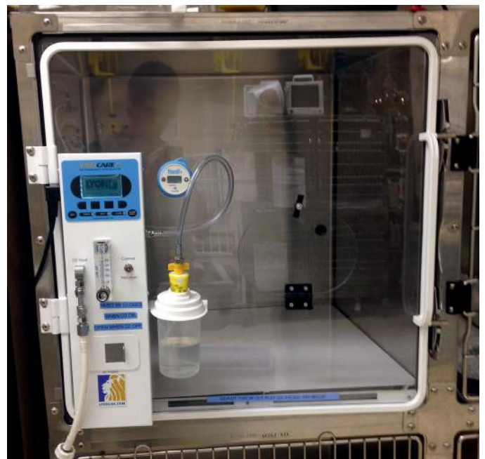
FIGURE 8-16 Pro-Care Therapy door (Lyon Electric). This therapeutic door allows the transformation of a regular hospitalization cage into an ICU cage with oxygen and heat support.
