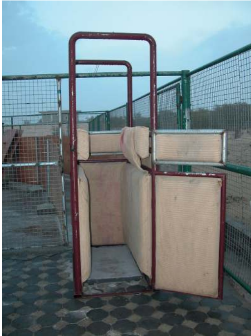
FIGURE 6-4 Custom-built restraining device specifically designed for subadult and adult ostriches ( Struthio camelus ). This device is made up of a frame built entirely with welded galvanized pipe of different diameters and walls and doors made up using \frac{3}{4} inch- (19 mm-) thick marine plywood screwed to the frame. The interior walls and doors are padded using high density 3 inch- (76 mm-) thick foam covered with commercial grade knitted shade cloth. The front and back upper doors are open or closed depending on the height of the ostrich and the type of procedure to be carried out. Please note the wide band fixed on the interior side of the device. This is made of the same shade cloth and is used as a restraining belt to stop the ostrich from jumping.
