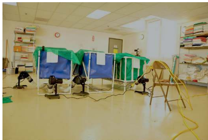
FIGURE 10-41 Modified pet driers are used to blow warm air into net-bottomed pens to provide thermal support to oiled or freshly washed birds. (Oiled Wildlife Care Network, 2000.)
