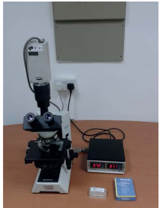
FIGURE 15-22 A more standard and less sophisticated system to evaluate semen samples. Such systems are commonly used in avian breeding centers to assess the quality of the spermatozoa before artificial insemination is carried out using freshly collected semen samples. The system is integrated with a warm plate, on which glassware can be preheated and samples can be temporarily placed before examination. The microscope is provided with a heated stage and a video camera connected to a monitor for observation of the type and quality of the movement of the spermatozoa.
