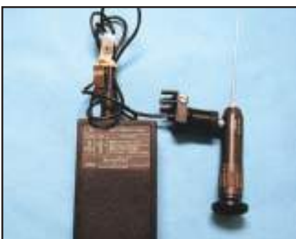
Fig 1.16e | The final scope with battery pack for full mobile endoscopy. The author (GJH) uses it for tracheoscopy without anesthesia on canaries. This is a portable, lightweight field unit and it also produces more than enough light.
