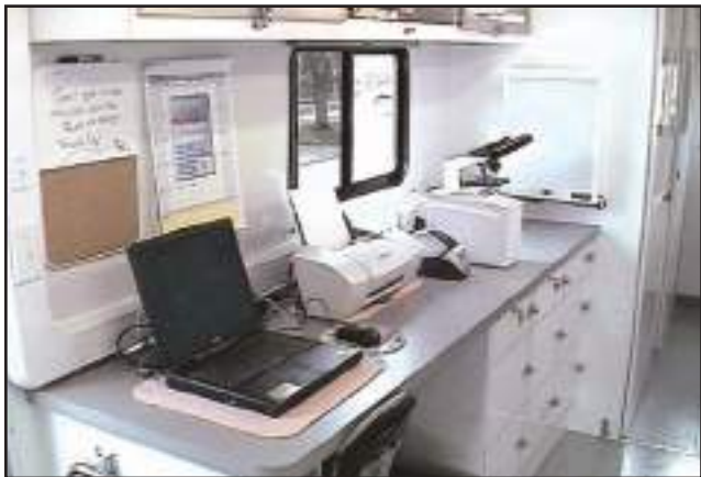
Fig 1.12b | Miniature laptop computers and compact equipment powered by generators, batteries or plugging into an outside source allow all laboratory procedures to be performed.
