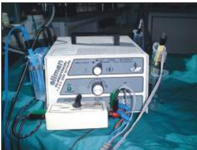
Fig 35.7c | This unit has been modified to allow multiple bipolar or unipolar hand pieces with a flick of a switch.
