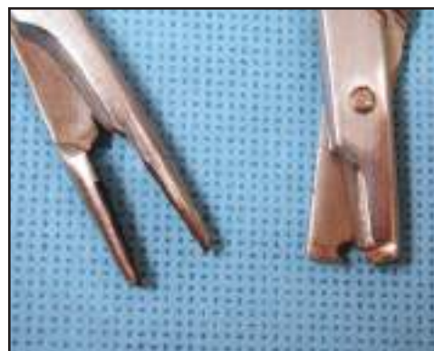
Fig 1.32c | The flat grind wheel on a hand-held rotary tool ® can be used to remove the needle holder's tips and make the cuts shown in Fig 1.32d. This makes an excellent band remover for the fine plastic bands and some aluminum bands used for birds like canaries.
