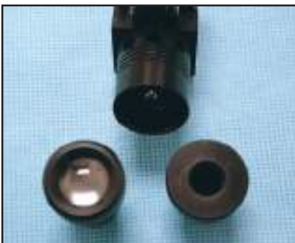
Fig 1.16b | Close-up of removed lens (left) and the custom-made adapter (right) to allow this unit to power an endoscope.
