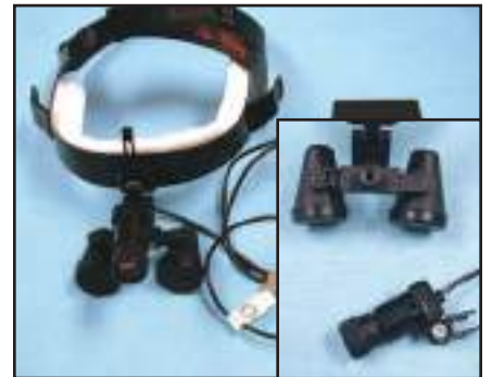
Fig 1.16a | Steps to custom power an endoscope for portability. The embedded magnification focus lens is removed from over the light of a Surgitel magnification scope.
