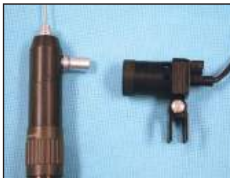
Fig 1.16c | The modified light is ready to be attached to the endoscope.
