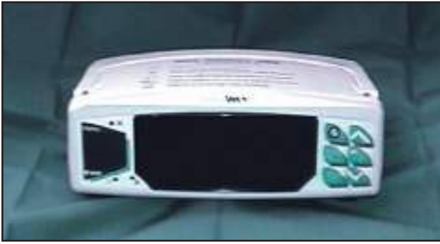
Fig 33.14 | Several manufacturers offer combination anesthesia monitoring equipment such as this pulse oximeter and ECG instrument f .
