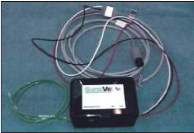
Fig 33.12 | ECG probe f with adapter. This adapter box connects standard ECG leads to the esophageal probe.
