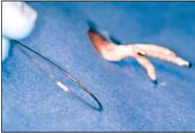
Fig 34.2 | Titanium pin bent past 180°.
