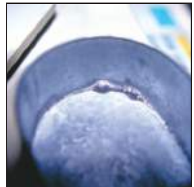
Fig 6.21c | Lead soldered galvanized water dish.
