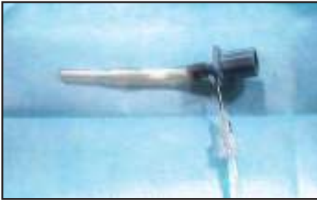
Fig 33.8 | Cole endotracheal tube shortened to reduce dead air space. The endotracheal tube adapter has been modified to allow the attachment of a side stream capnograph. This has been accomplished by mounting an 18-ga needle into the lumen of the adapter with the needle bevel facing the patient.
