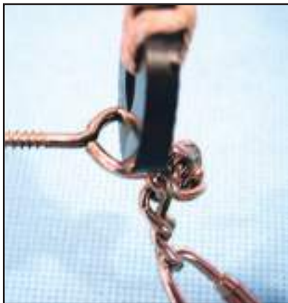
Fig 6.19b | Toys are frequently made of polished galvanized metal. Here a magnet is used as a diagnostic tool — if it attaches, the underlying metal is iron. This is a common metal that is galvanized to prevent rust. Galvanization is primarily zinc. The circular shaped magnet has attached to a chain and anchor screw, indicating galvanization is likely and these objects should be removed.
