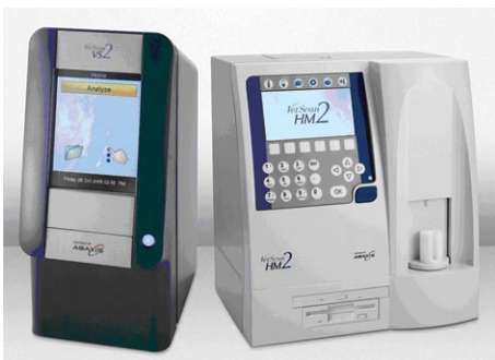
Fig 4.1 Technical advancements have led to the development of plasma chemical analysis machines that can run samples on the very small volumes of blood that can be collected from even the smallest avian patient. (Photo courtesy of Abaxis North America, Union City, CA, USA)
