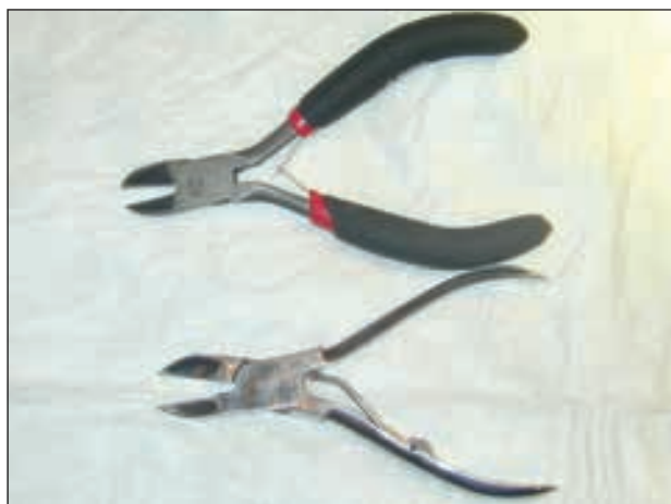
15.16 Wire cutters or small pliers should be used for wing trimming in order to cut the calamus sharply, to avoid splitting the feather.
