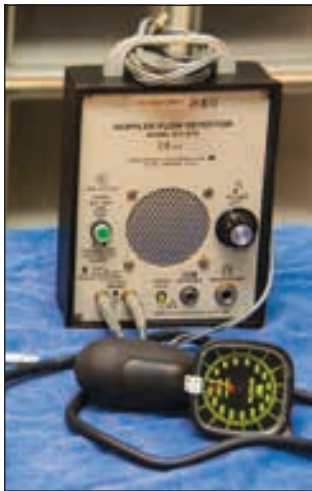
16.7 The use of a Doppler ultrasound pulse monitor is invaluable when monitoring patients under anaesthesia. It provides continual 'hands-free' audible monitoring of the pulse of the patient. The Doppler monitor also facilitates the intraoperative monitoring of indirect blood pressure, further augmenting patient monitoring acuity. (Reproduced from BSAVA Manual of Canine and Feline Nephrology and Urology )
