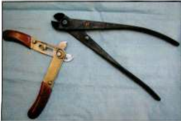
6.21 Ring cutters. The lower pair has a notch to prevent ring twisting and can be used for all but stainless steel rings. The upper pair is much heavier, with a sharp cutting edge; the grips are shaped to allow easier use. This pair can be used to cut some stainless steel rings.
