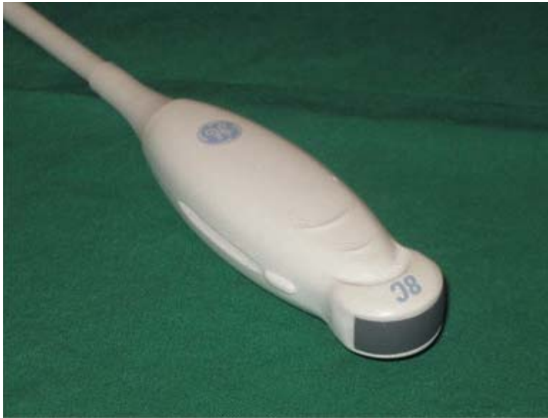
Fig. 1-43: Transducers used on birds for ultrasonography examinations should have a small coupling surface. This micro-curved probe with a frequency of 7.5 MHz is ideal for the examination of birds up to a body weight of 2 kg.
