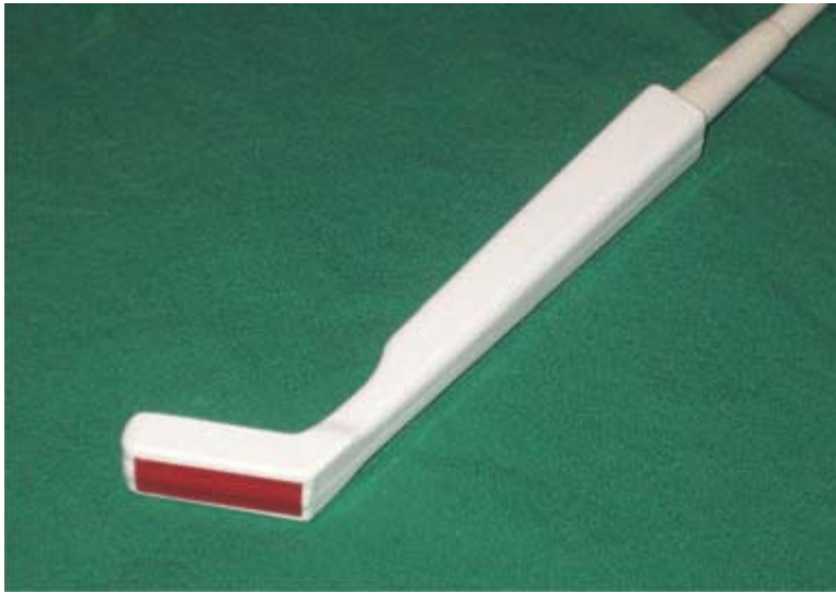
Fig. 3-33: Special transducers such as this hockey stick allow the use of sites which cannot be reached with a standard transducer. This transducer can even be placed, without difficulty, in the prefemoral window of small chelonians.
